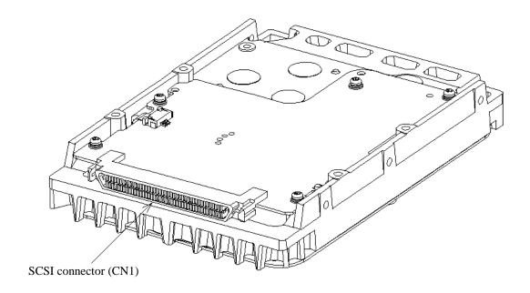
Figure 4.21 Connectors location of MC model
